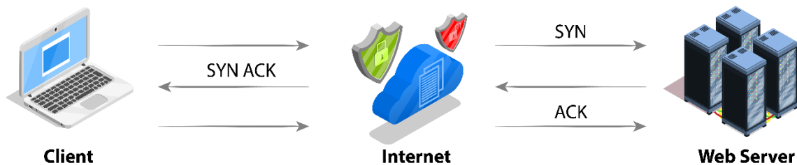
Gambar 42 TCP Threeway Handshake
